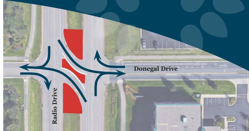
*Safety improvements at the Radio Drive and Donegal Drive intersection will eliminate left-turn movements from Donegal Drive to Radio Drive.*
